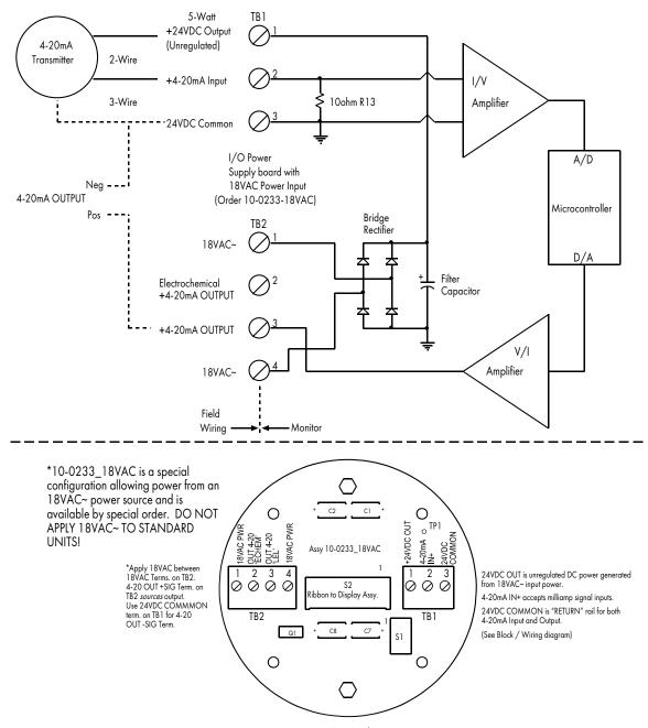
Figure 7-2: 10-0233-18VAC Block / Wiring Diagram
