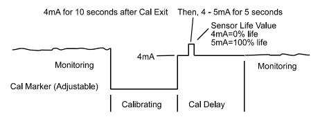
Figure 5-5: Transmit Sensor Life Timing Diagram
