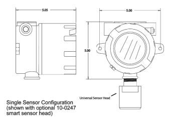
Figure 2-2: SenSmart 3000 Explosion-Proof Housing
