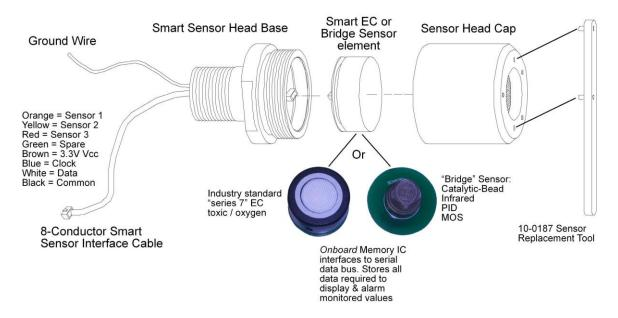
Figure 2-9: 10-0247 Smart Sensor Head Assembly
