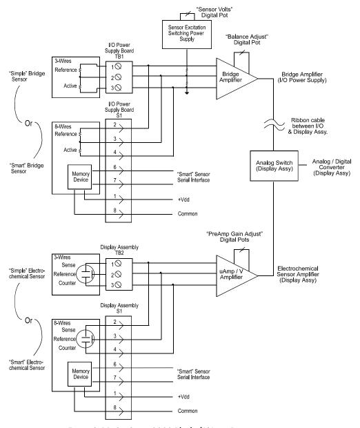
Figure 2-11: SenSmart 3000 Block / Wiring Diagram
