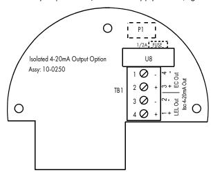
Figure 2-8: 10-0250 Isolated 4-20mA Output Option
