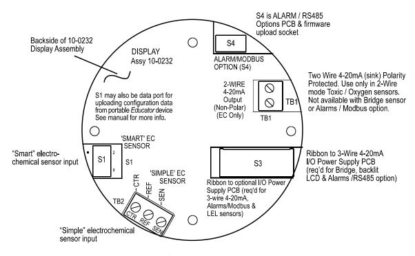
Figure 2-4: 10-0232 Display / SenSmart 2000 2-Wire 4-20mA Assembly
