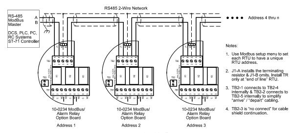
Figure 2-7: RS-485 Modbus Wiring
