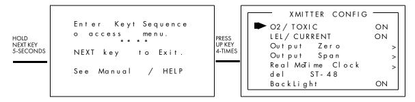
Figure 3-1: Transmitter Configuration Menu
