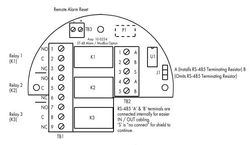
Figure 2-6: 10-0234 Alarm Relays / Modbus Option
