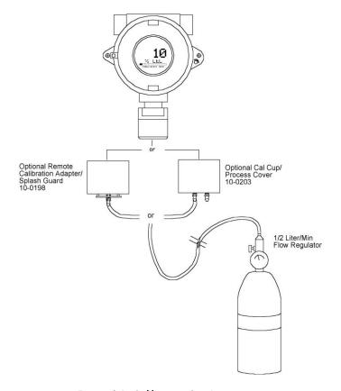
Figure 4-1: Calibration Gas Input
