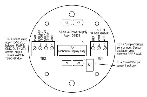
Figure 2-5: 10-0233 I/O Power Supply / 3-Wire 4-20mA Assembly
