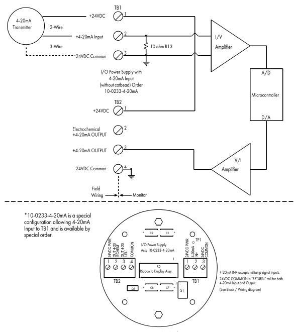
Figure 7-3: 10-00233-4-20mA Block / Wiring Diagram
