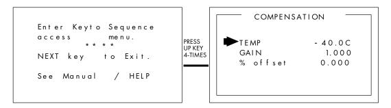
Figure 5-4: Temperature Compensation Menu
